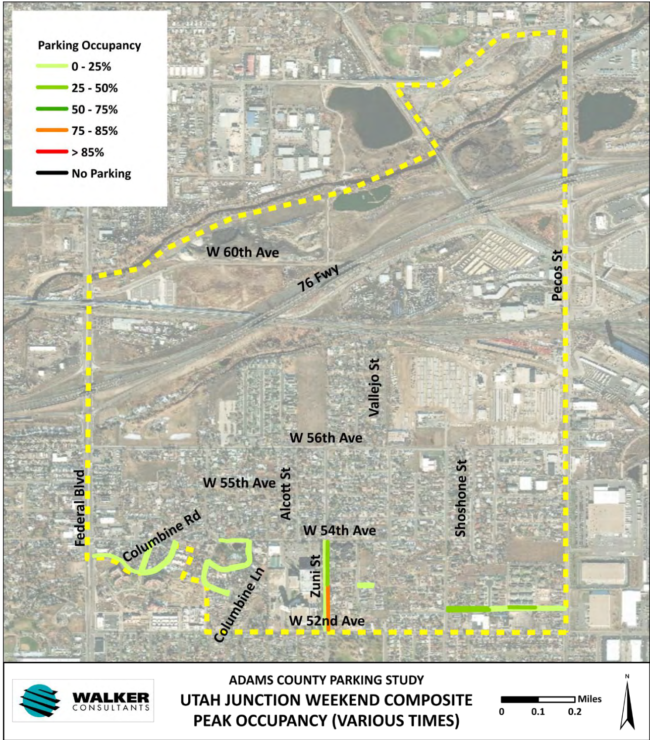
Figure 78: Utah Junction Heat Map of Localized Weekend Peak Occupancy by Block Face (Varying Times of Day)
