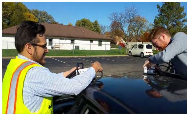
A PEO/PA attaching LPR cameras to a car roof with magnets
