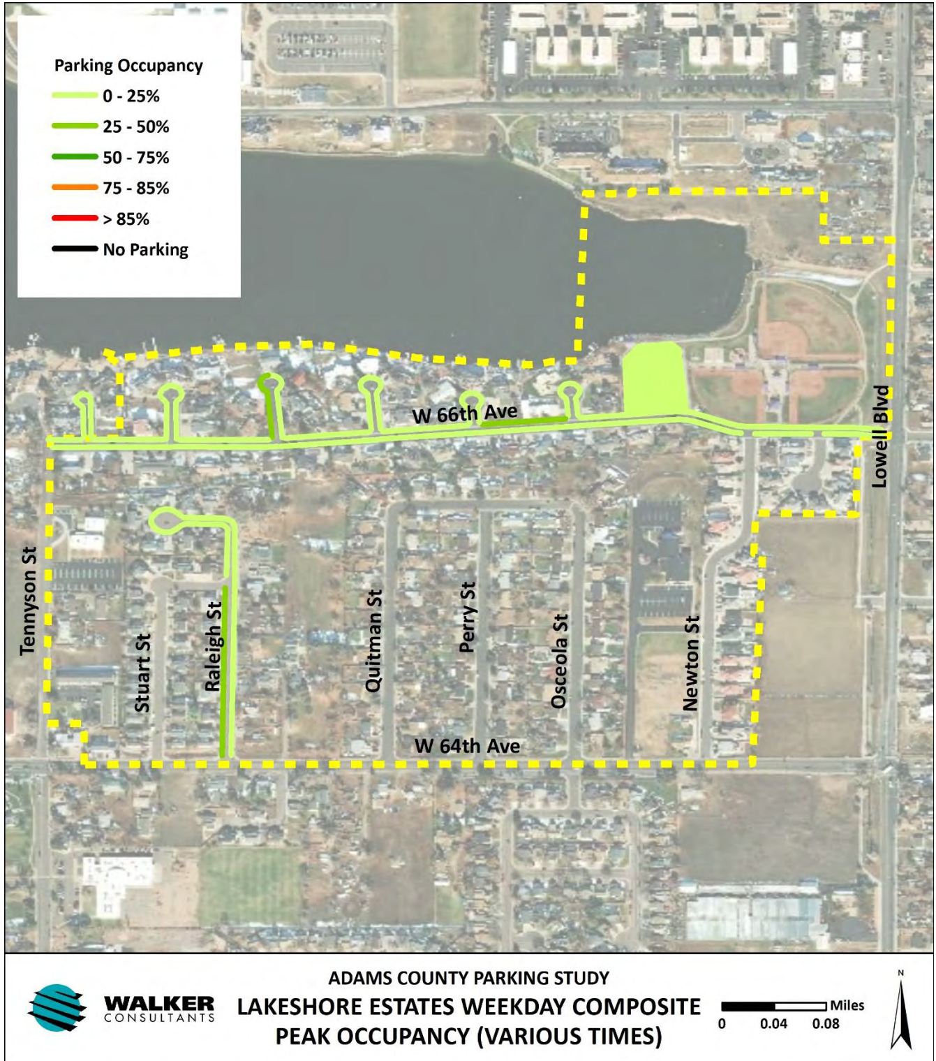
Figure 48: Lakeshore Estates Heat Map of Localized Weekday Peak Occupancy by Block Face (Varying Times of Day)
